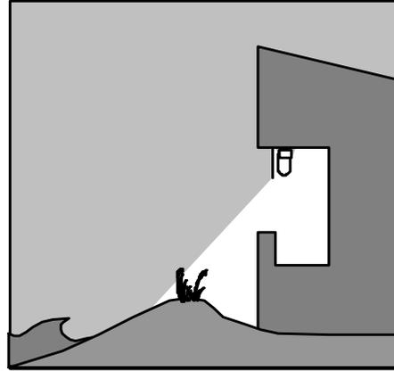
Completely shielding fixtures with a sheet of metal flashing can reduce stray light reaching the beach.
