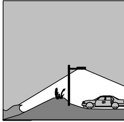
Fixtures with 90-degree cutoff angles can reduce the amount of stray light reaching the beach.
